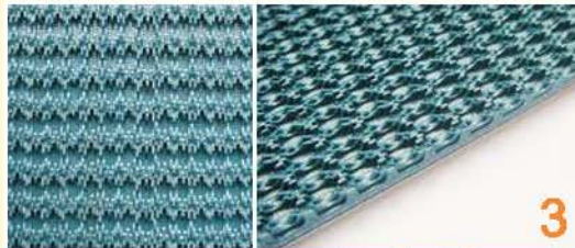
3 Name: Rough top(Super grip) Thickness: 2.4mm Property: Incline conveying, very high friction Application: Logistic ,Airport .
