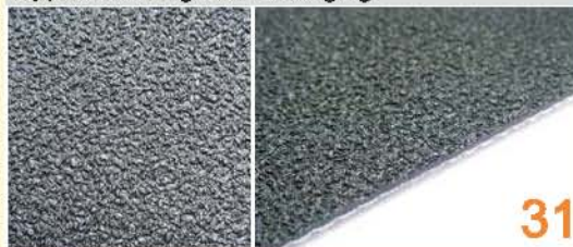
Name: Sandblast Code: 31 Thickness: 0.2mm Width: 2000mm Property: Non adhesive surface medium friction Application: Logistic Treadmill belt Roller wrapping
